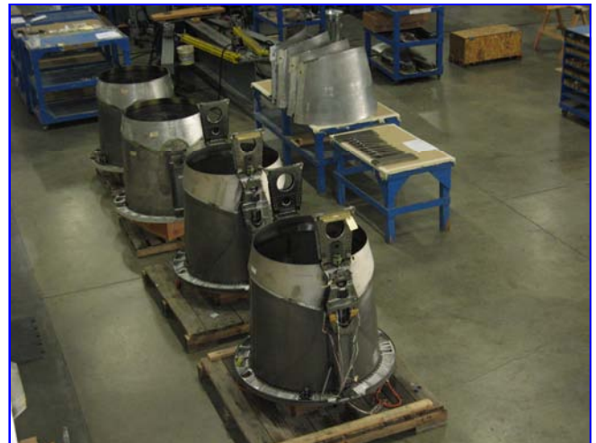
On-going Construction of Dugan Kinetics EP-80 Thrust Reverser Assemblies at Soloy's Olympia Facility.
