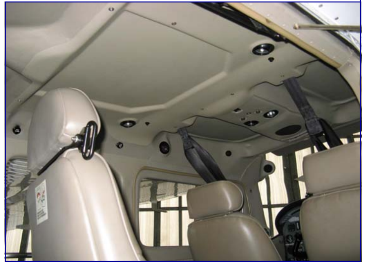
Re-contoured Headliner Modification with 4-Point Pilot/Copilot Shoulder Harnesses
